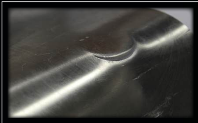
* Image shows full penetration of the aluminiums plate
